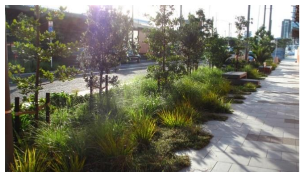
Figure 8: Bioswales could be located in streetscapes to improve the water quality in the precinct
