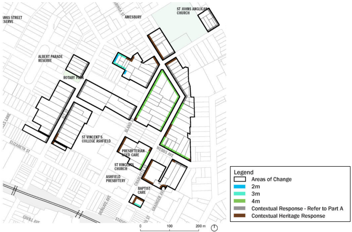
Figure 58: Northern Spine – Building Setbacks
