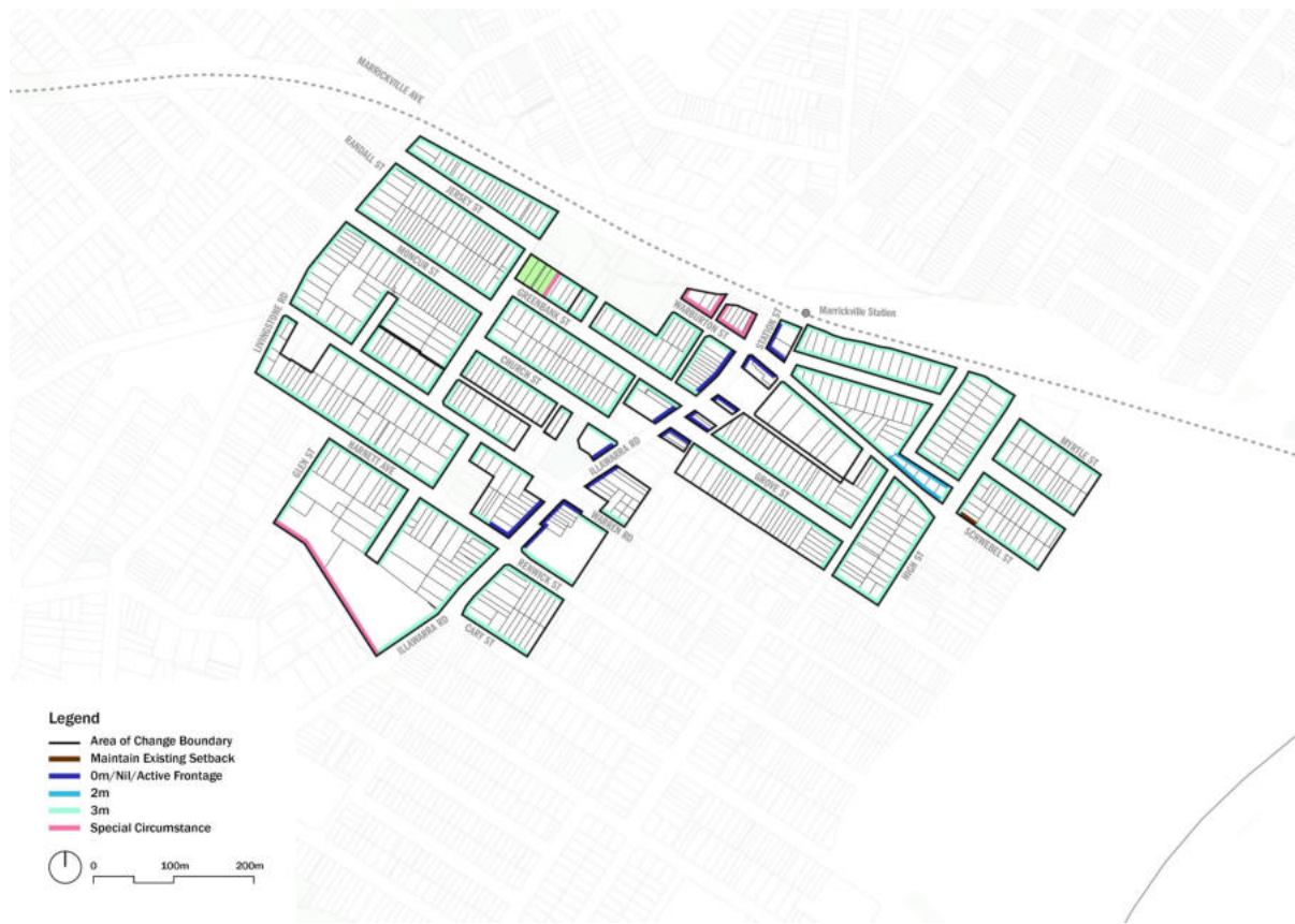
Figure 13: Illawarra Road Marrickville – Building Setbacks
