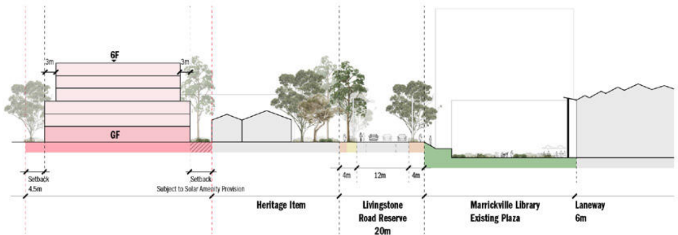
Figure 33: Section 1 - Through Livingstone Road
