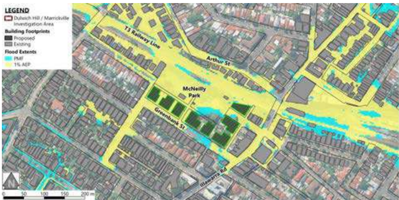
Figure 8-37 Flood extents near Uplift Location FF
