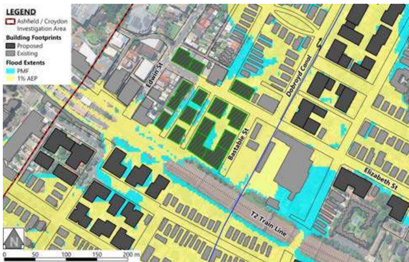
Figure 8-7 Flood extents near Uplift Location B
