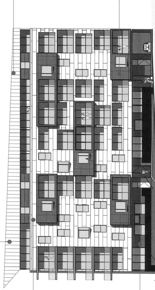
Render paint finish to prefab. concrete walls Colour Dulux Monk P-GTG6
