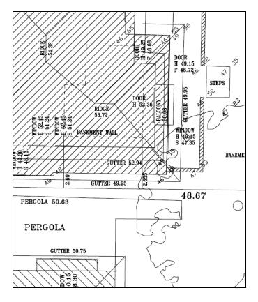
Figure 1 survey plan location of basement indicated broken lines showing distacne from boundary 2.69m & 2.655m
