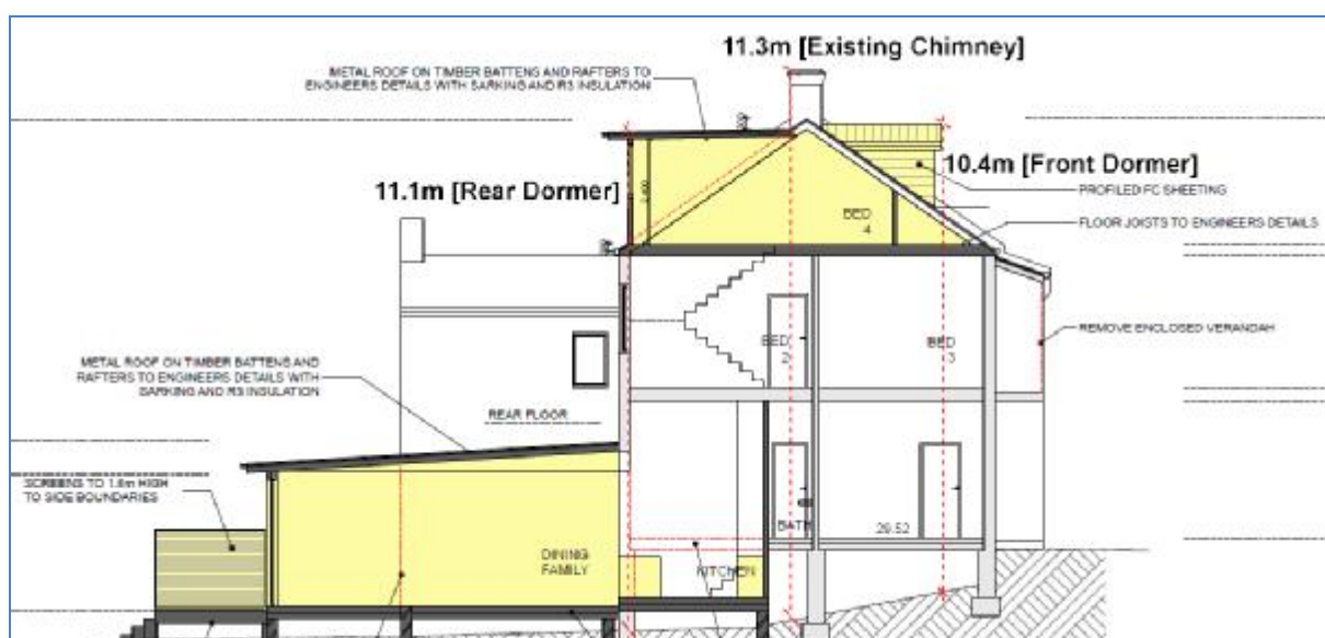
Image 1: Non-compliance with building height standard
