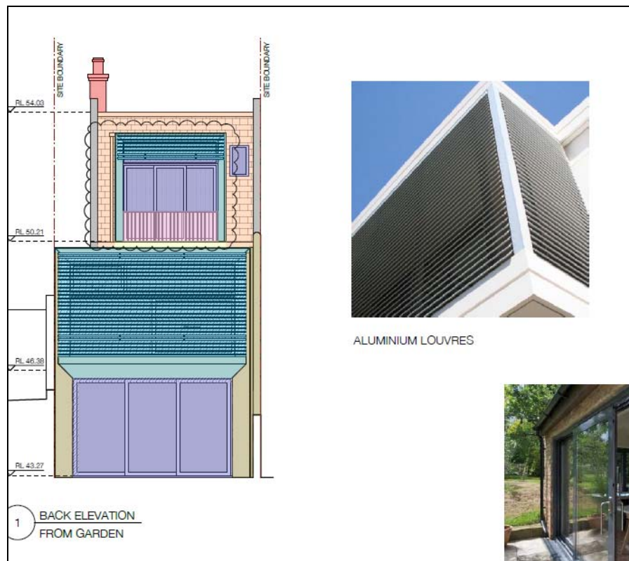
Image 16: Approved Rear Elevation showing metal louvers – No.94 Douglas Street, Stanmore
