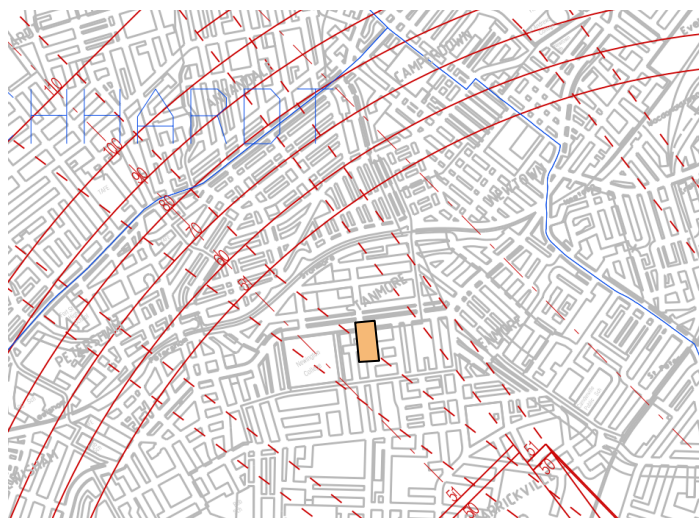
Figure 14: Extract from the Obstacle Limitation Surface contour map for Sydney Airport as it applies to the site
