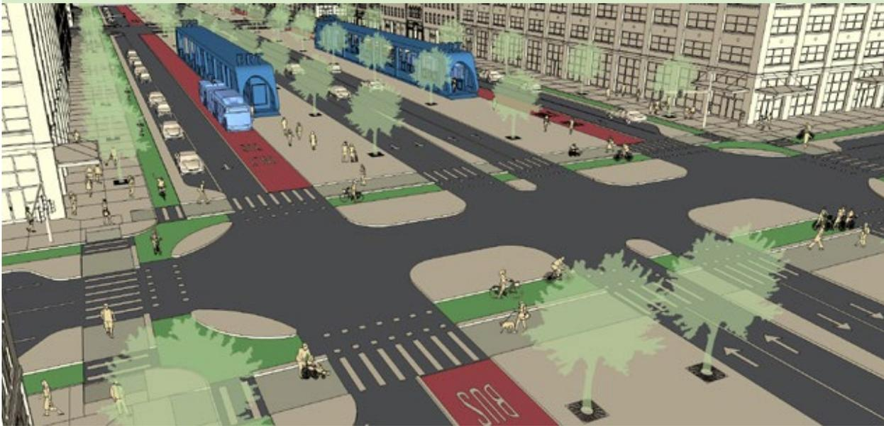
**EXAMPLE OF A BUSWAY ALIGNED TO THE INNER CURB OF THE SERVICE ROAD ON A BOULEVARD-TYPE STREET WITH A CENTRAL ROADWAY AND PARALLEL SERVICE ROAD**
