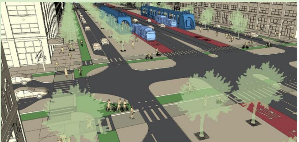
**EXAMPLE OF A BUSWAY ALIGNED TO THE OUTER CURB OF THE CENTRAL ROADWAY ON A BOULEVARD-TYPE STREET WITH A CENTRAL ROADWAY AND PARALLEL SERVICE ROAD**
