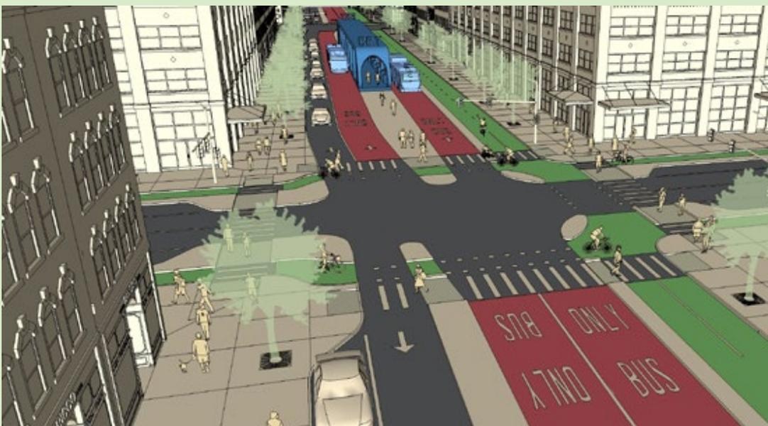
**EXAMPLE OF A BUSWAY THAT RUNS TWO-WAY ON THE SIDE OF A ONE-WAY STREET**
