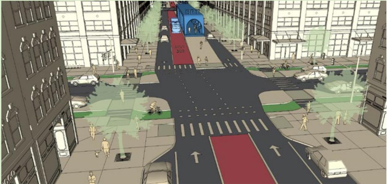
**EXAMPLE OF A BUSWAY CENTRALLY ALIGNED ON A ONE-WAY STREET**
