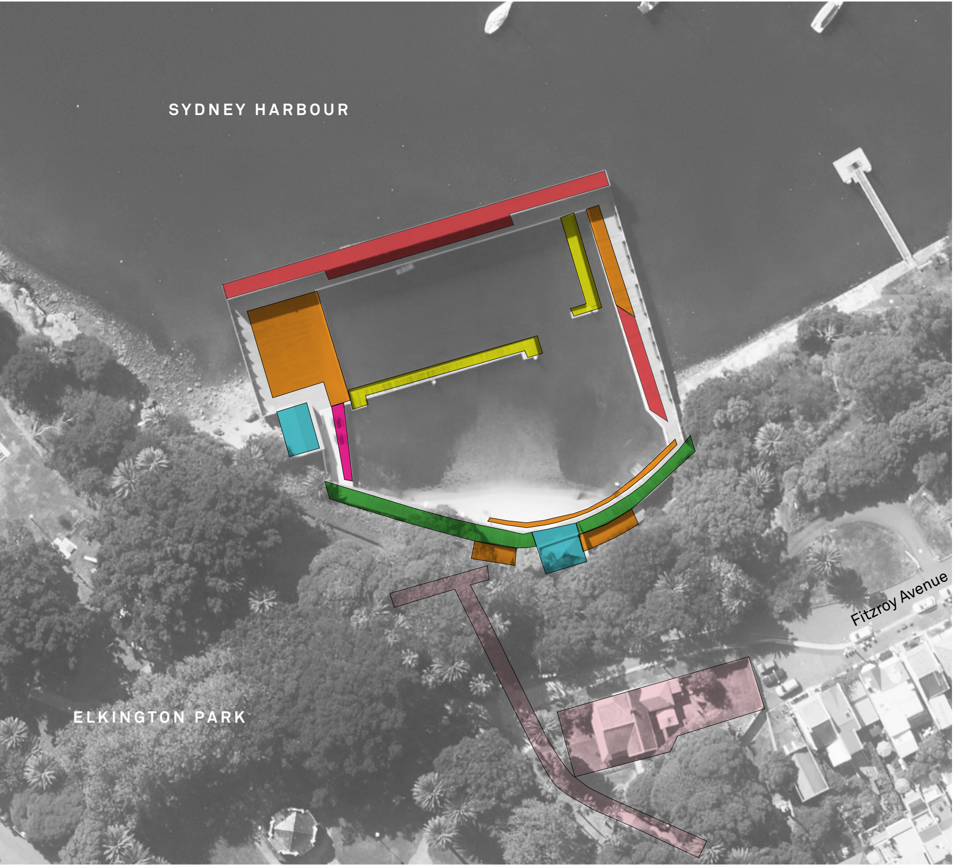
Diagram of the different construction period for the existing Baths structure
