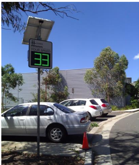
Figure 7.2: Radar speed display
