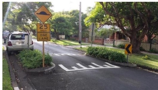
Figure 7.8: Single lane road hump with planted kerb extensions
