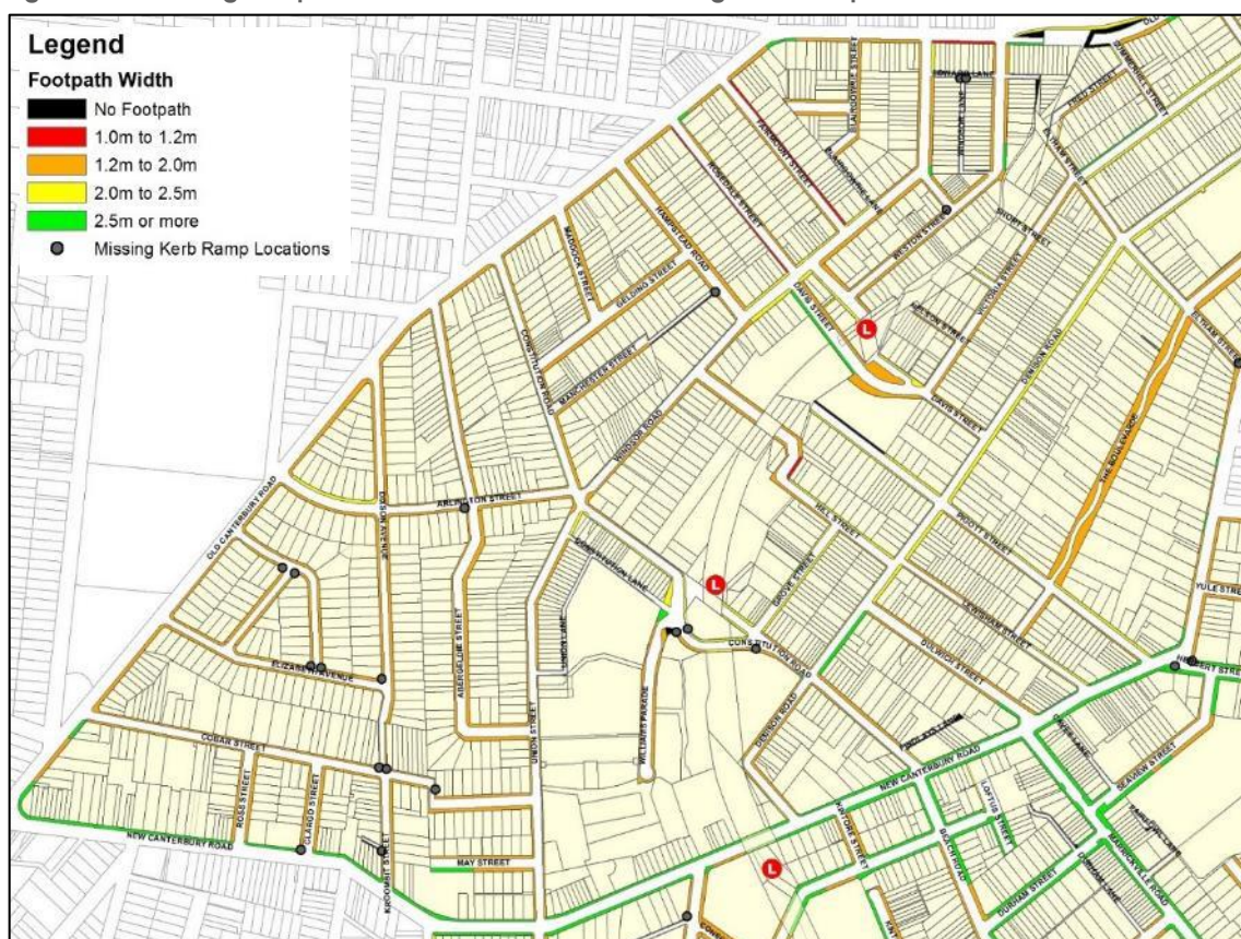
Figure 3.7: Existing Footpath Network & Locations of Missing Kerb Ramps
