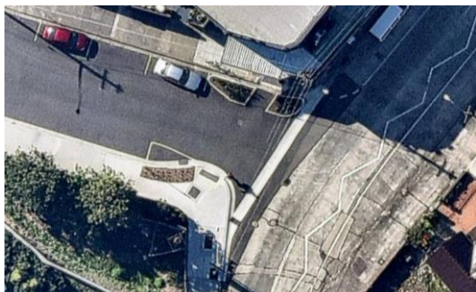
Figure 7.3: Entry Treatment – Kerb Extensions
