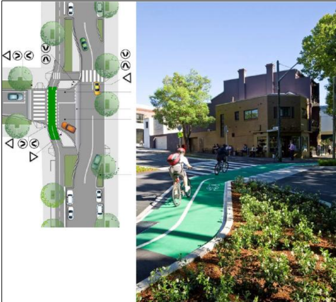
Figure 4-1 Bend Out Intersection Treatment
