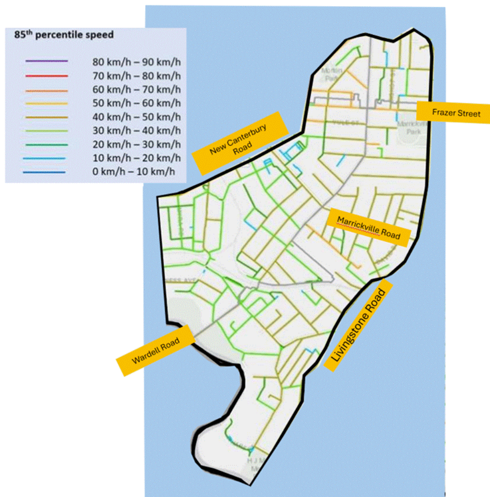
Figure 3 85 th Percentile Speed Profile for Area 8
