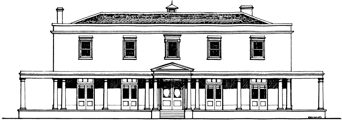
GARRY OWEN: c1840. A conjectural drawing which shows the house as it might have been. No evidence of any colonnade or pediment has been found but the main entry doorway architrave and cornice, and the interior Greek Revival details, suggest that something more than a post and beam verandah was intended. A timber post and striped corrugated iron verandah existed after the house was converted for patients in 1876.
