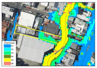
Figure 6. Flood Hazard (H1-H6) Existing Conditions – 1% AEP Flood
