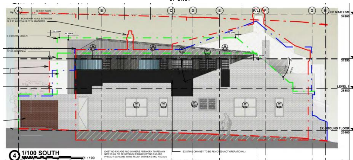
Figure 6: excerpt of DA23 D Elevations, South Elevation (Eton Lane) showing proposed addition and increasing of height to rear.
