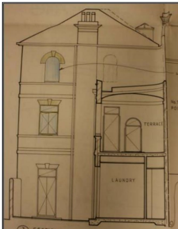
Figure 3.17 1991 amendments showing proposed deletion of the concrete balustrade from the trio of windows on the second floor of the Bates Street elevation (below) and proposed new openings on the western elevation.
