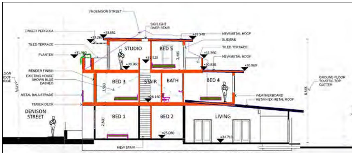
Figure 6 - No. 76 Denison Street Section Diagram as Approved under DA201400210
