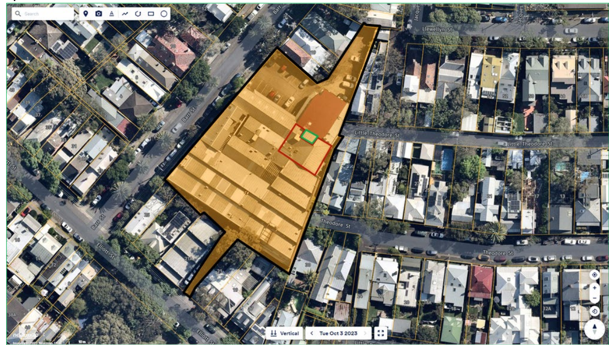
Figure 1: General shape of the mixed-use building, black border, at 1-15 Barr Street, Balmain. Approximate location of Unit F14. In red border is the roof demolition to be replaced with a raised roof, and in green border, is the proposed roof demolition to be left open.
