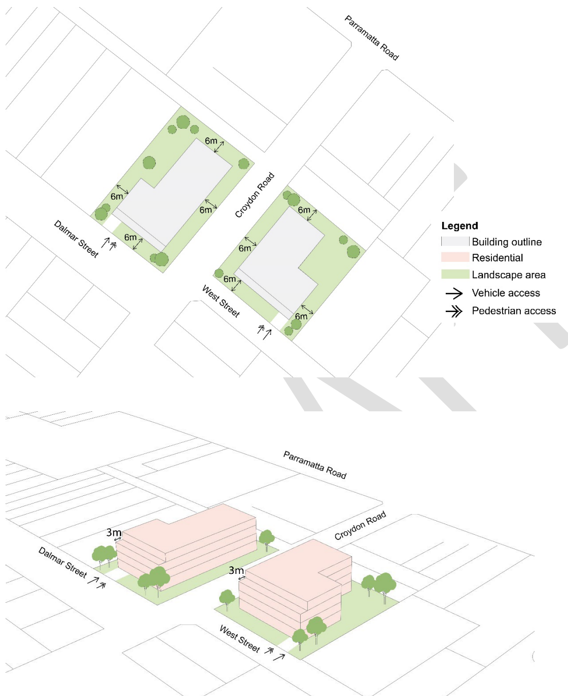
Figure 14: Indicative Type 1C – Narrow Lot Infill Croydon Road corner – storeys, building envelope, scale and site layout requirements – plan and axonometric views
