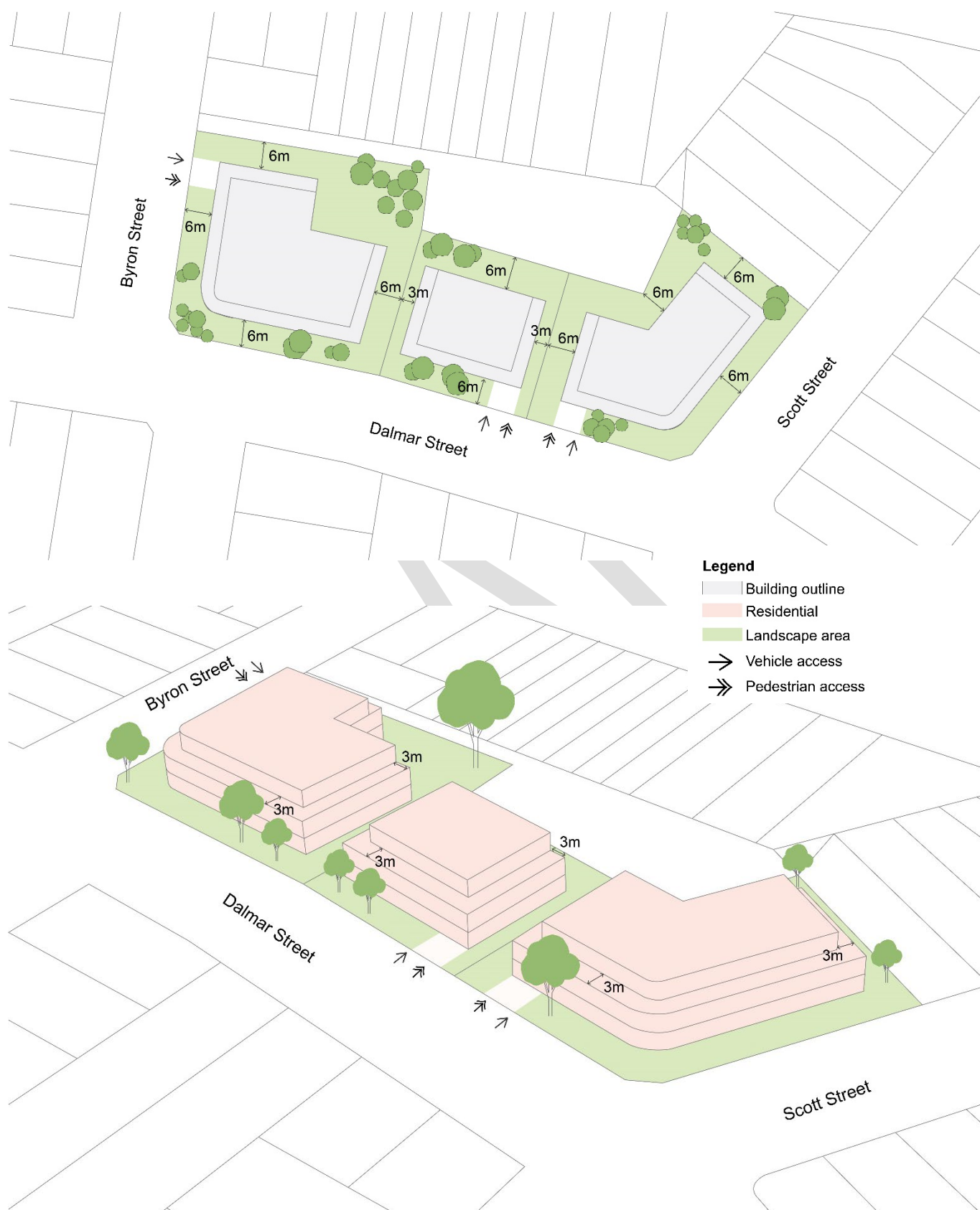
Figure 15: Indicative Type 2 Row House – storeys, building envelope, scale and site layout requirements – plan view and axonometric views
