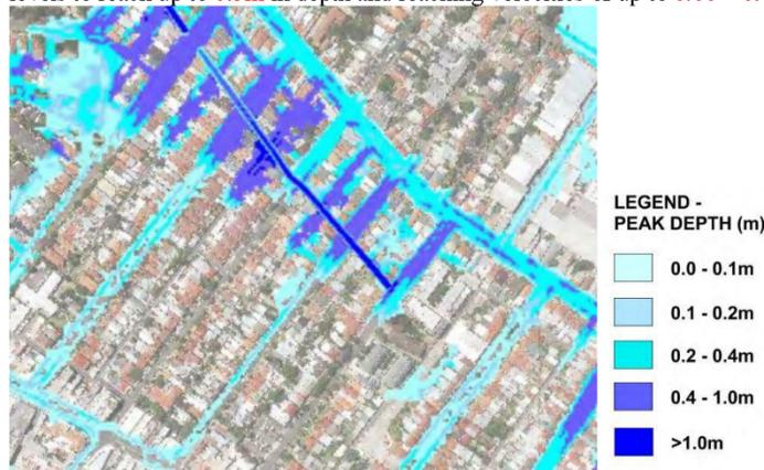
Figure 3 - Flood Levels for 1% AEP
