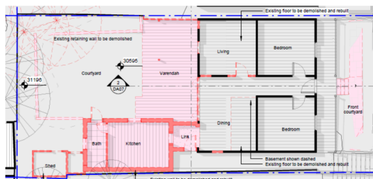
Figure 13: demolition plan, ground floor
