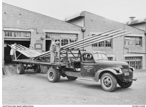
Employees of F Dickin Ltd loading the rear spar for transport c.1945. Milton Kent photographer. (Australian War Memorial)
