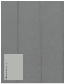
ALUMINIUM HORIZONTAL CLADDING - ULTRACLAD SHADOWLINE WEATHERBOARD FIRST FLOOR ADDITION DULUX - SHALE GREY
