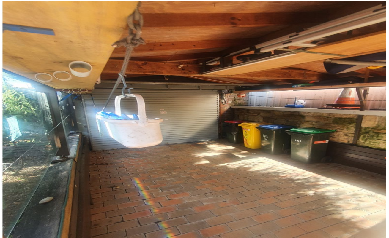
Figure 4: the existing carport which will be demolished. The floor level of the carport is indicative of the depth of excavation at the subject site to allow for the proposed rumpus and landscaped area. Source: site inspection 18.05.2022.
