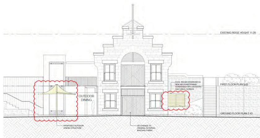
Figure 56: Extract of BJB Architects proposal plans, East elevation showing both the proposed outdoor seating/dining area to the south side of the building and the proposed air conditioning condenser with acoustic and visual screen to the north side of the building.
