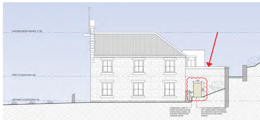
Figure 57: Extract of BJB Architects proposal plans, North elevation showing the proposed air conditioning condenser with acoustic and visual screen. The proposed bin enclosure is located behind the existing sandstone wall marked with a red arrow and will not be visible when approaching the site from the north.
