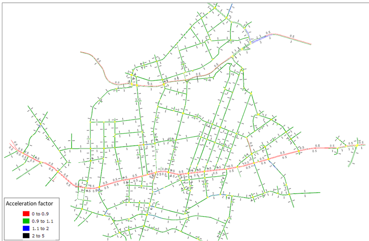
Figure 1: Acceleration factor visualisation of the road network
