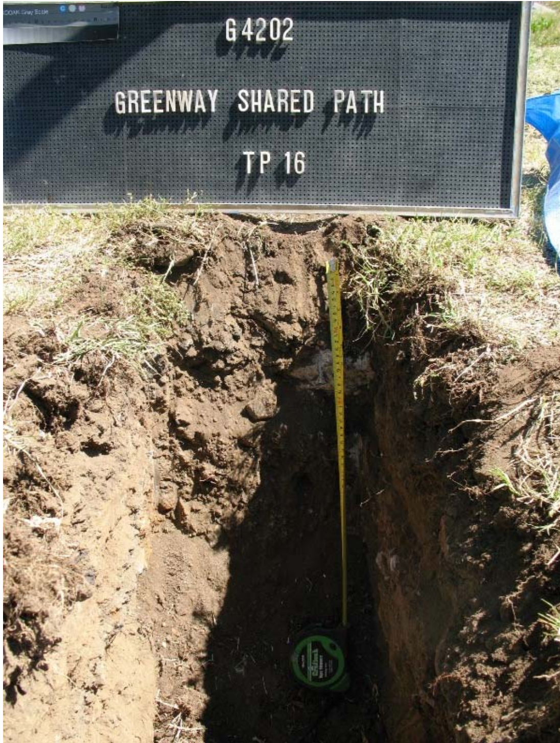
Test Pit 16 (tape extended to 500mm)
