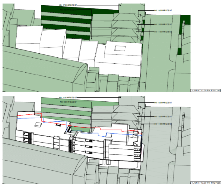
Figure 10: Solar Access Diagram Existing vs Proposed 12:30pm Source: Benson McCormack Architecture
