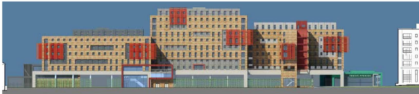
Eastern elevation of the site in its context showing entrance/exit to the one-way services road and separation of the plant room from the rest of the site.
