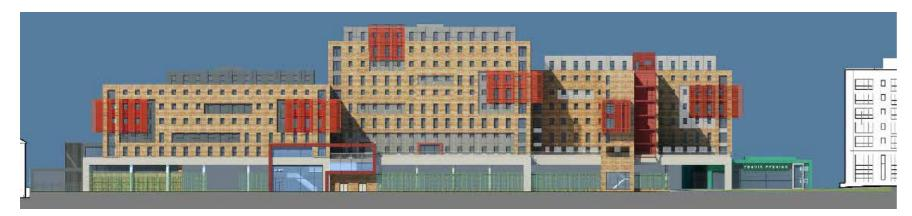
Eastern elevation of the site in its context showing entrance/exit to the one-way services road and separation of the plant room from the rest of the site.
