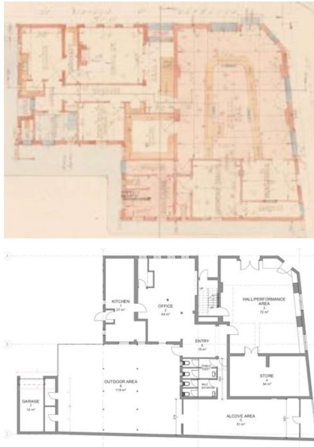
Figure 7.1 Comparative plans of original and current layout showing the extent of change
