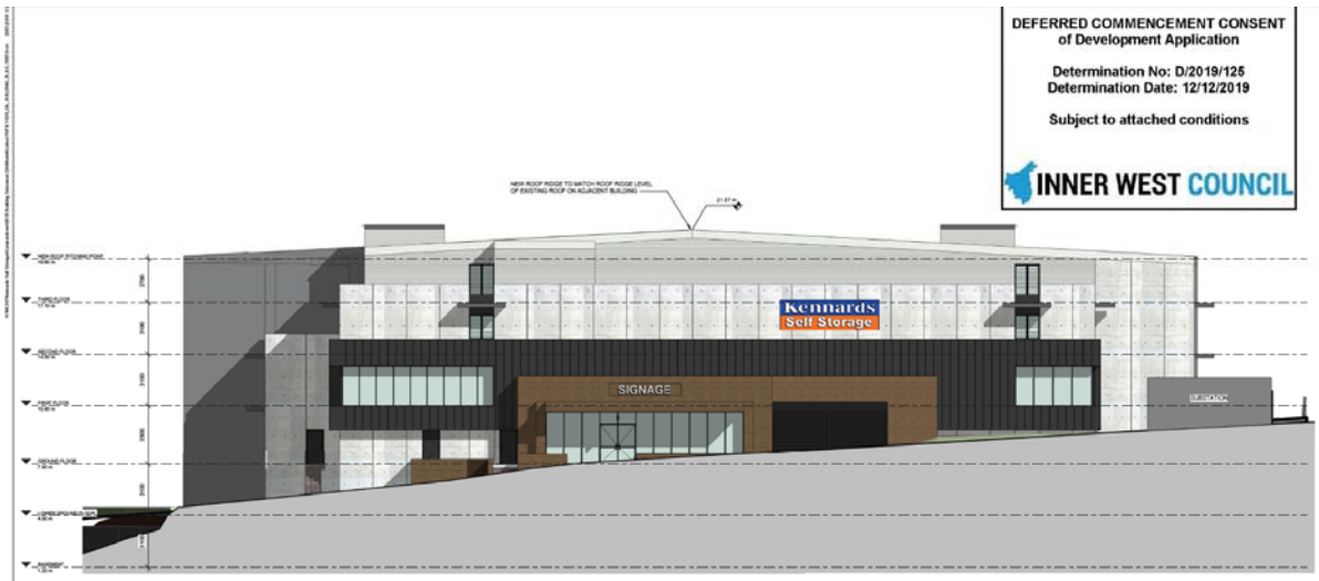
Figure 19- West Elevation to Chester Street (the existing 5 storey main building will have a new 6 storey extension) as approved D/2019/125 - 1-19 Booth Street, Annandale
