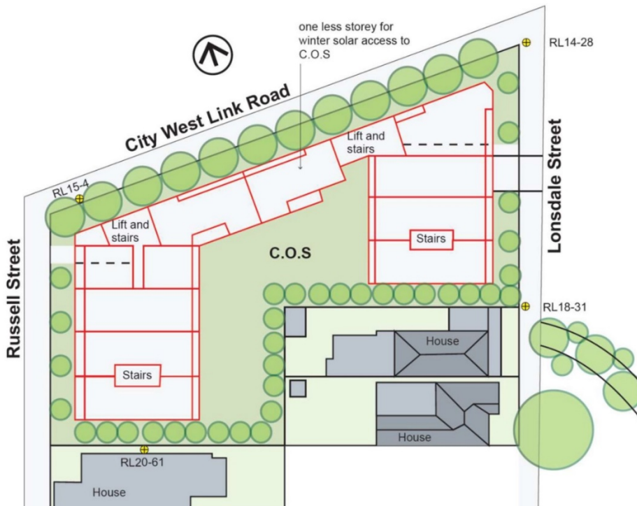
Figure 6: Indictive site layout option 1 complying with proposed FSR and HOB. (Source Council Officers)
