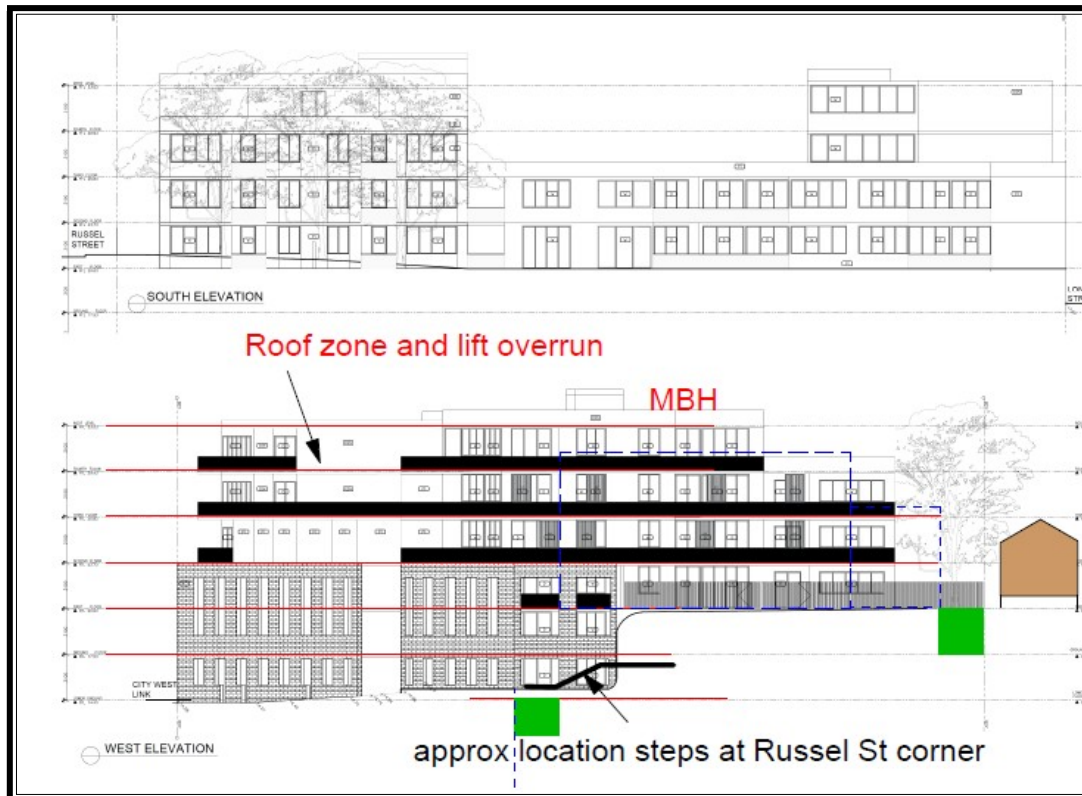
Figure 20: Council's concept design with a 1.5:1 FSR and reduced height to RL 33.2 (Source: annotated over DRA drawings by Council Urban Designer)
