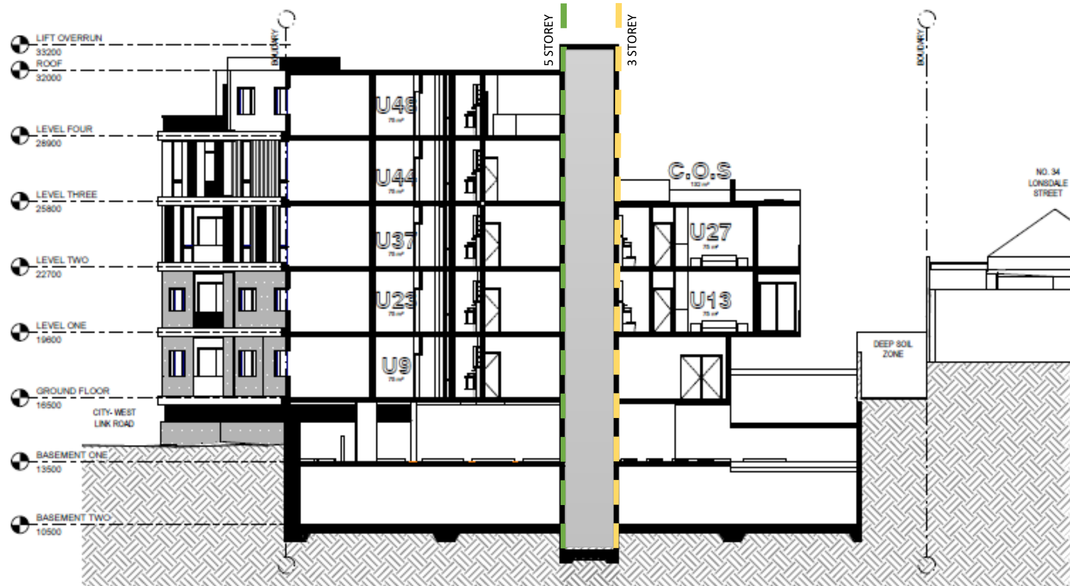
Figure 3F.4 Within the same site, minimum separation should be shared equitably between buildings. On sloping sites, appropriate separation distances ensure visual privacy for apartments on different levels
