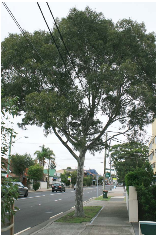
Figure 4.7 - The installation of ABC cabling above street trees is an excellent way to achieve medium sized trees while maintaining the health, vigour and form of the trees. Formative pruning can achieve appropriate branching structures well before the lines are reached. This is a successful example of trees and ABC on the north side of Gardeners Road, in Rosebery (Photo - Arterra)
