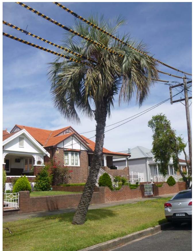
Figure 4.6 - The installation of ABC cabling above street trees may assist with retaining trees that may otherwise need to be heavily pruned or removed as a result of power line clearances. (Example - Martin Street, Dobroyd Point) (Photo - Arterra)
