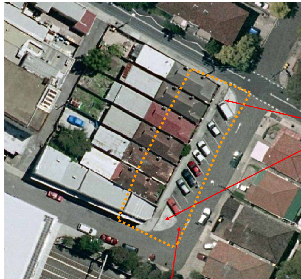
A catchment area of approximately 1,100 m 2 , 100% impervious can be diverted into the raingarden on Wood St. The raingarden area available is up to 20 square metres. The treated water would need to be discharged back to the gutter downstream of the raingarden.
