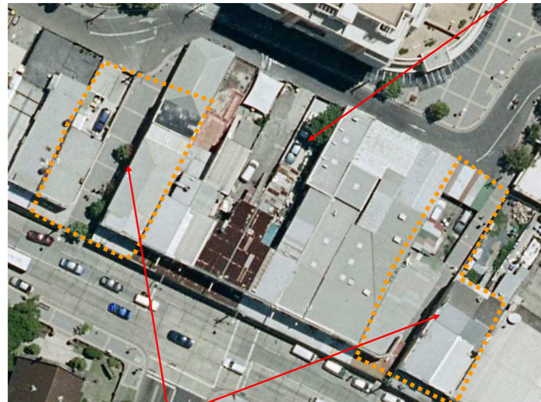
The catchment area that can be treated in each lane varies from lane to lane, but typically is best undertaken when the roof water from the adjacent building can be incorporated into the hydraulic design of the raingarden.
