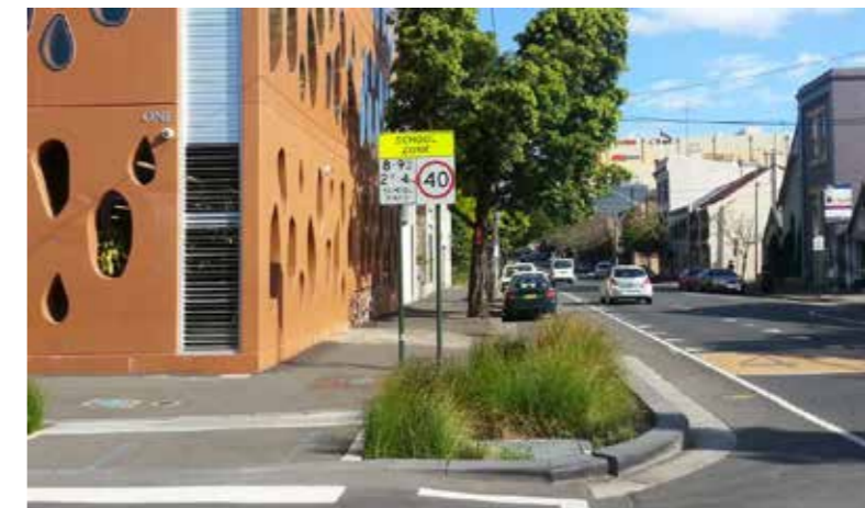
An example of a similar streetscape raingarden incorporated into the road pavement is shown in Bay St Ultimo. The raingarden is treating the road and adjacent roof drainage runoff before discharging the water back to stormwater. The additional cost to incorporate a raingarden into a street planter garden is relatively low and.
