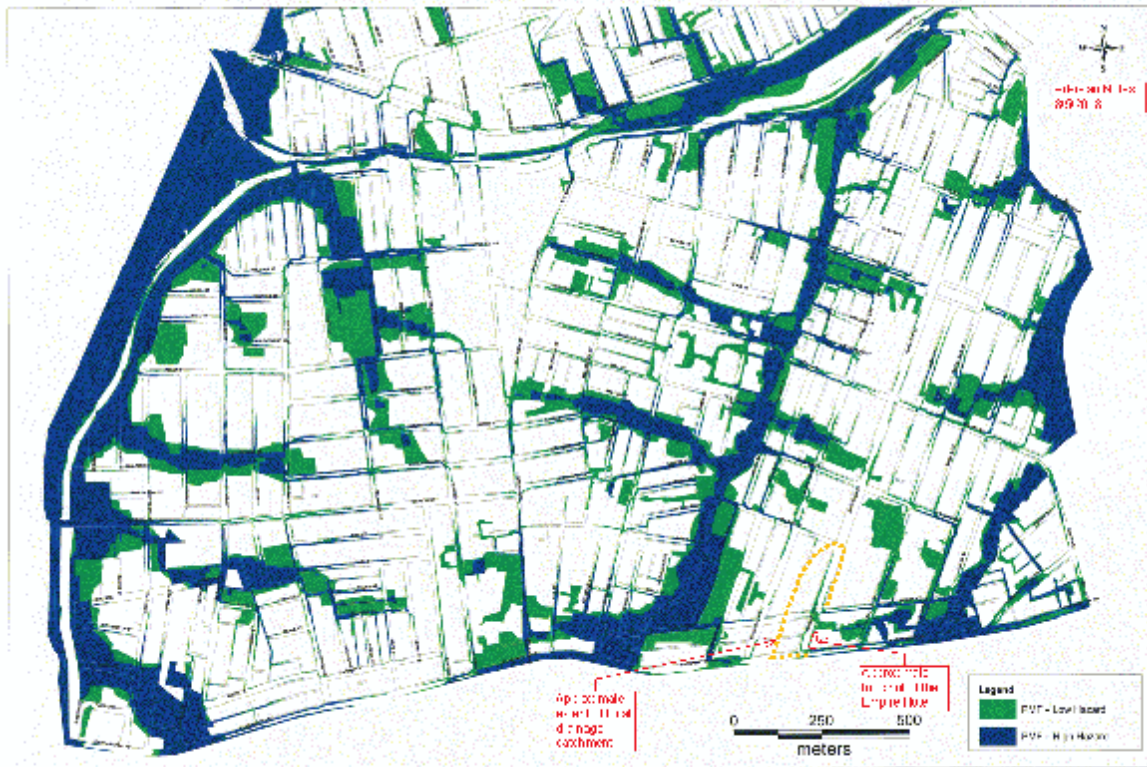
Figure 9.3 - PMF - Hazard Sheet 1 Leichhardt Flood Study 2019/2020 Leichhardt Flood Study Figure 9.3 - PMF - Hazard Sheet 1
