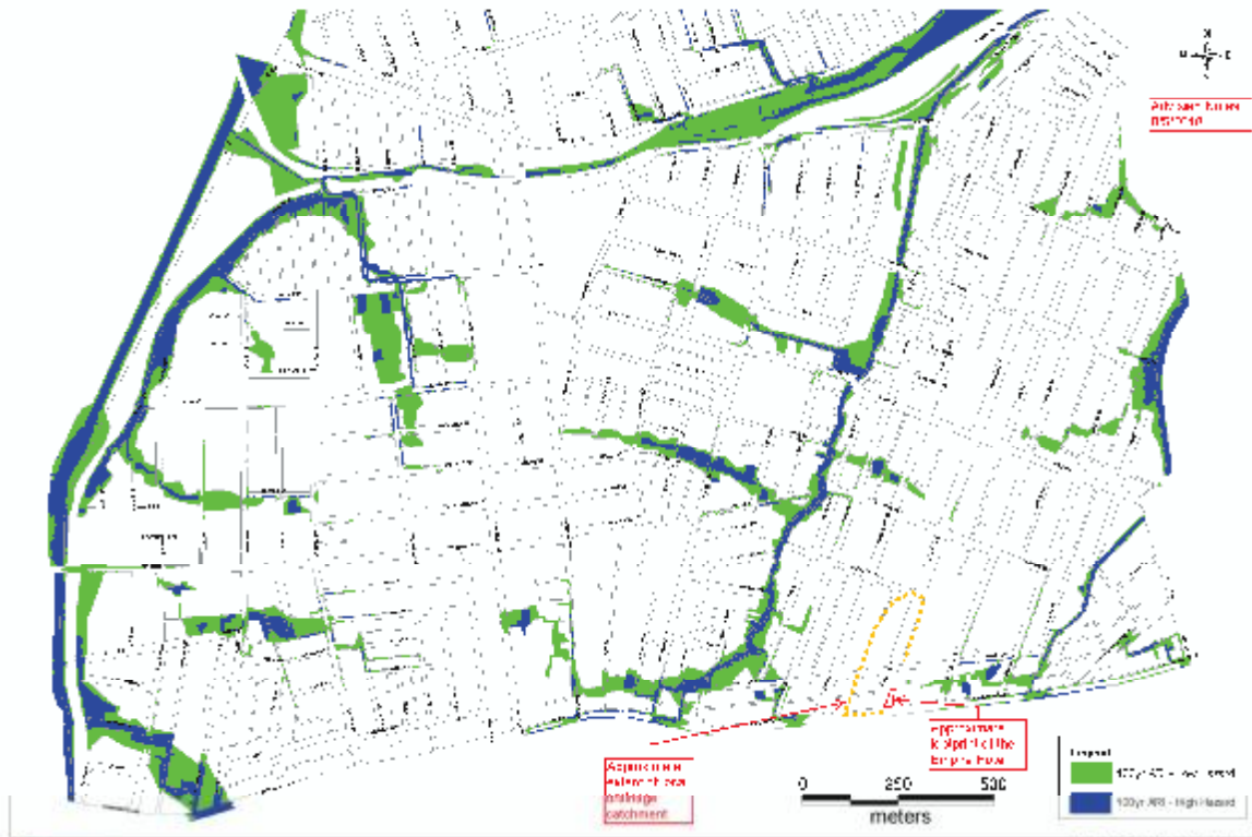
Figure 9.2 - 100yr ARI - Hazard Sheet 1 Leichhardt Flood Study 2019/2020 Leichhardt Flood Study Figure 9.2 - 100yr ARI - Hazard Sheet 1
