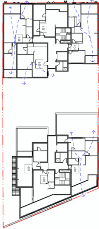
Plan 3 2ND FLOOR PLAN - CROSS VENTILATION 1:200
