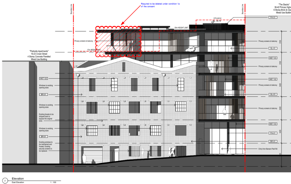
Picture 2 – East Elevation Plan - indication of Building B elements required to be deleted by condition 1a of the consent.
