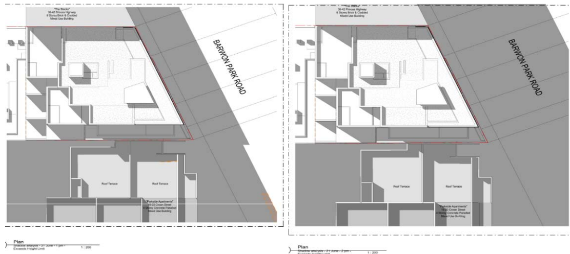
Picture 6 – Extent of shadow cast by height variation detailed in orange – image to the left is solar access for neighbouring roof top terraces at 1pm, image to the right is solar access for neighbouring roof terraces at 2pm
