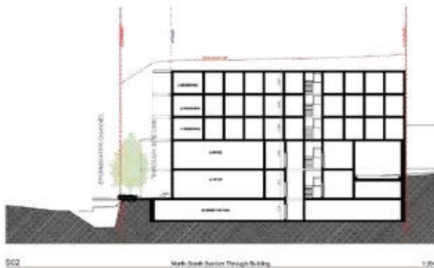
Figure 8 - North-South Section through the building indicating 6m setback from the creek and 17m (5 storey) height limit
