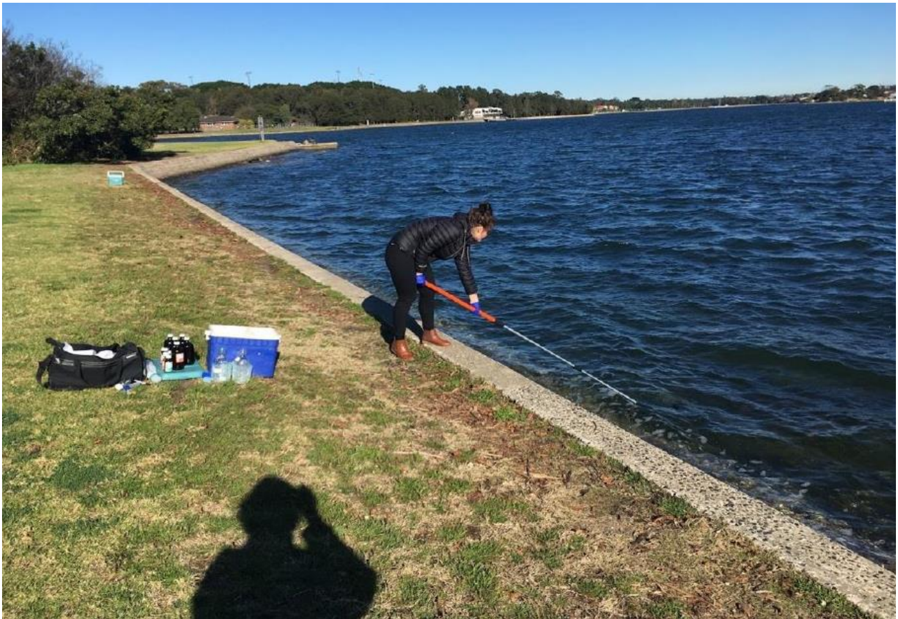
Figure 6: Shoreline surface water sampling (samples collected from 2 locations over 6 events)
