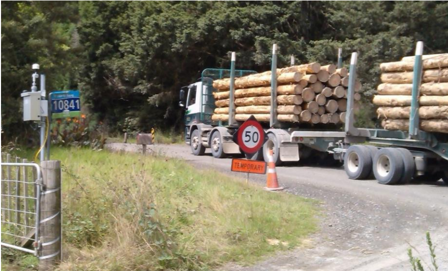
Figure 1 - A single dust monitor on the left measures emissions from an unsealed road
