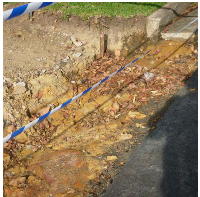
Figure 1.23 Learmonth St, Dobroyd Point - sandstone based soils that typically have shallow and impoverished soils with bedrock often impeding proper drainage. (Photo: Arterra)
