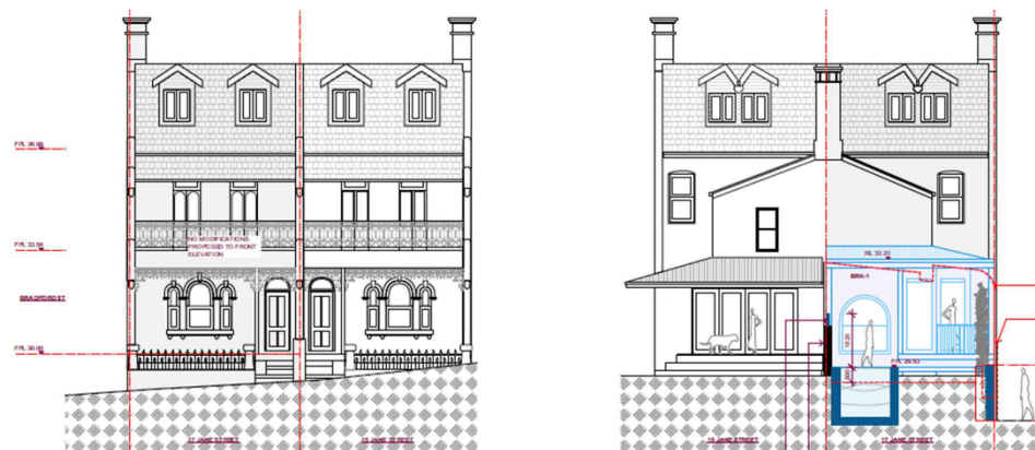
Figure 2 – Proposed front and rear elevations of the site and its neighbouring terrace at 15 Jane Street
