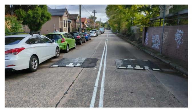
Shifting approx. 300mm to avoid construction joint Speed cushions to be installed to the same dimensions as the existing rubber cushions Replace signs due to damage, graffiti or missing (no posts)
